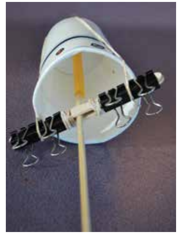
Kids can add binder clips to the plunger. When pulled back against the rubber bands, the added weight (i.e., mass) gives the plunger more potential energy, enabling it to do more work.
