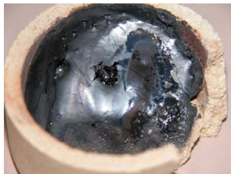
Slag, a low-oxygen by-product of Cardiff's device. Slag may prove useful as a raw material for bricks, pavement, or radiation shielding.
