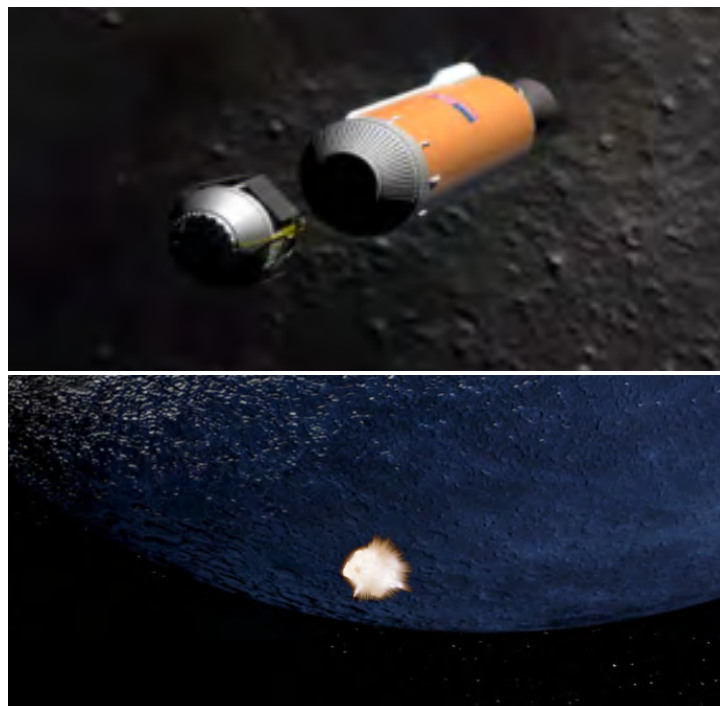
Top: LCROSS approaches the Moon. Bottom: The first of two impacts delivered by the split craft.
